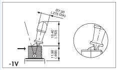
1 locked position (function 6) Typical angle of throw: 26°
