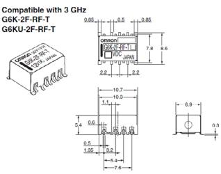
Note 1. Each value has a tolerance of  $\pm 0.3$  mm. Note 2. The coplanarity of the terminals is 0.15 mm max.
