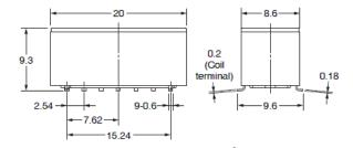
Note 1. Each value has a tolerance of  $\pm 0.3$  mm. Note 2. The coplanarity of the terminals is 0.1 mm max.
