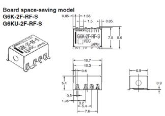
Note 1. Each value has a tolerance of  $\pm 0.3$  mm. Note 2. The coplanarity of the terminals is 0.15 mm max.
