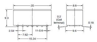
Note 1. Each value has a tolerance of ±0.3 mm. Note 2. The coplanarity of the terminals is 0.1 mm max.
