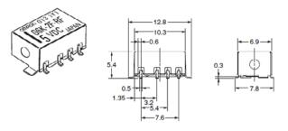
Note 1. Each value has a tolerance of  $\pm 0.3$  mm. Note 2. The coplanarity of the terminals is 0.15 mm max.
